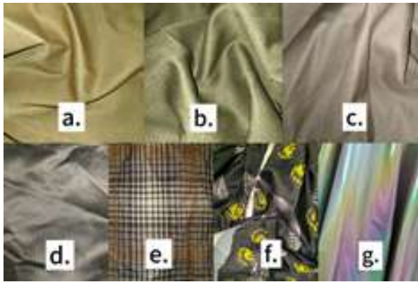
Gambar 7. Material bahan : katun toyobo kuning (a), katun toyobo hijau (b), katun toyobo khaki (c), kain taffeta (d), kain tartan (e), kain digital printing (f), kain hologram (g).
