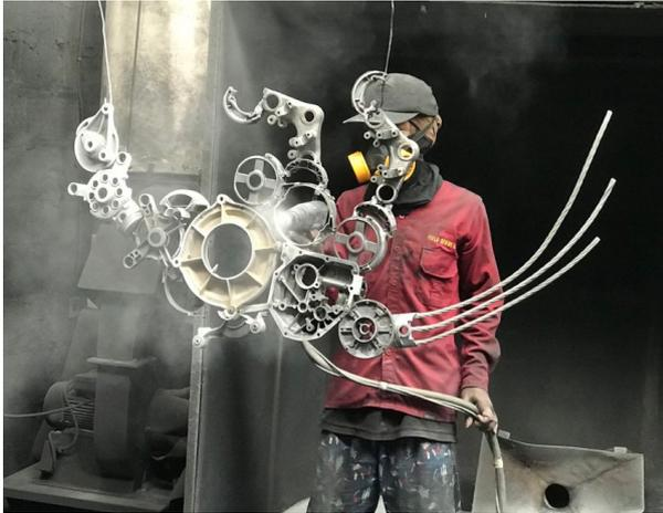
**Gambar 12. Proses powder coating**
