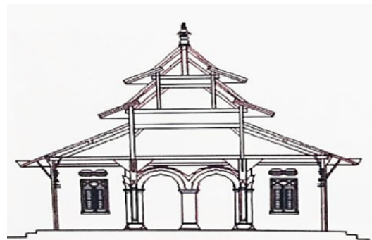
Picture 6. The Overlapping roof with three Steps. (Source : Author 2020)
